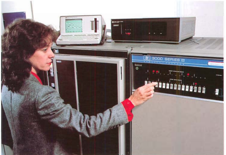
The HP 4951A protocol analyzer, at left on the HP 3000 computer, offers high-performance test capability.
