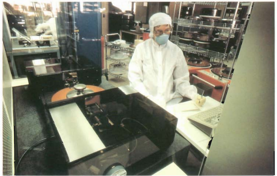
A traditional clean room requires workers to keep dust levels low by wearing gowns, masks and gloves.
